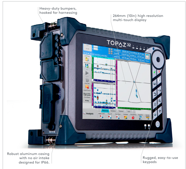
Figure 1: Annotated breakdown of TOPAZ32 showing its key features.
